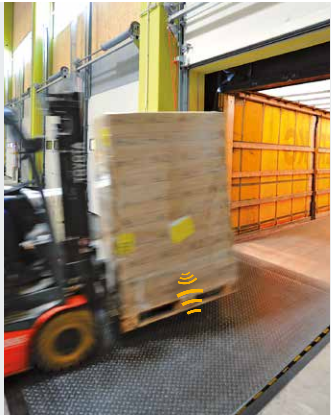
Automatic recording of goods movements, simply while crossing the dock leveller.
